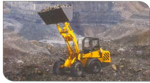
Hydrostatic drive with automotive control, 2 stages shiftable under load, single lever (Joystick) for drive and working hydraulics control.
