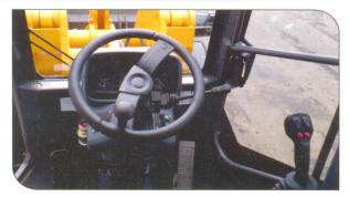
Hydrostatic steering,  $+/-40^{\circ}$ Maximum steering angle Turning radius (Over rear end) 3780 mm
